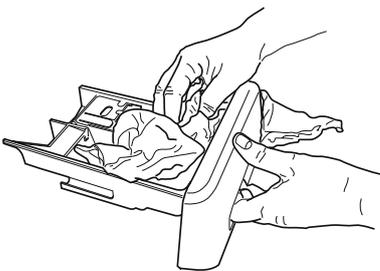
5. Reinstall the detergent dispenser and push it back into the detergent compartment.
