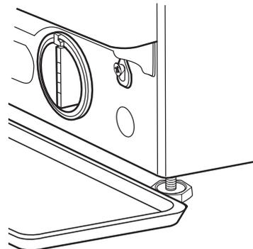
3. Drain the water: slowly turn the filter counter-clockwise until all the water has come out. Allow the water to flow out without removing the filter. Once the container is full, close the water filter by turning it clockwise. Empty the container. Repeat the procedure until all the water has been drained.
