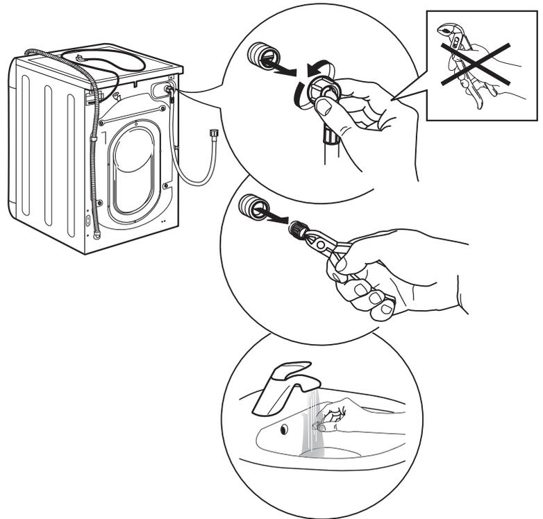
4. Insert the mesh filter again. Connect the inlet hose to water tap and washing machine again. Do not use a tool to connect the inlet hose. Open the water tap and check that all connections are tight.
