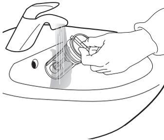
6. Insert the water filter and reinstall the plinth:
