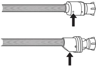
For water stop hoses: check the small safety valve inspection window (see arrow). If it is red, the water stop function was triggered, and the hose must be replaced by a new one.
