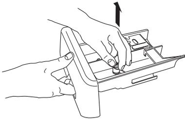
3. Clean all parts under running water, removing all detergent or softener residues.
