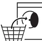
Open the door and load the laundry. Load the articles one at a time loosely into the drum, without overfilling. Observe the load sizes given in the "PROGRAMME CHART" table. Overloading the machine will result in unsatisfactory washing results and creased laundry.
